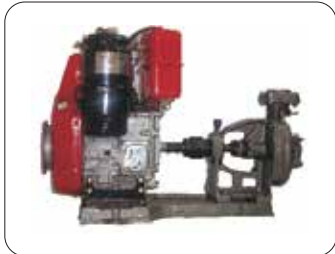
DIESEL ENGINE PUMP SETS
